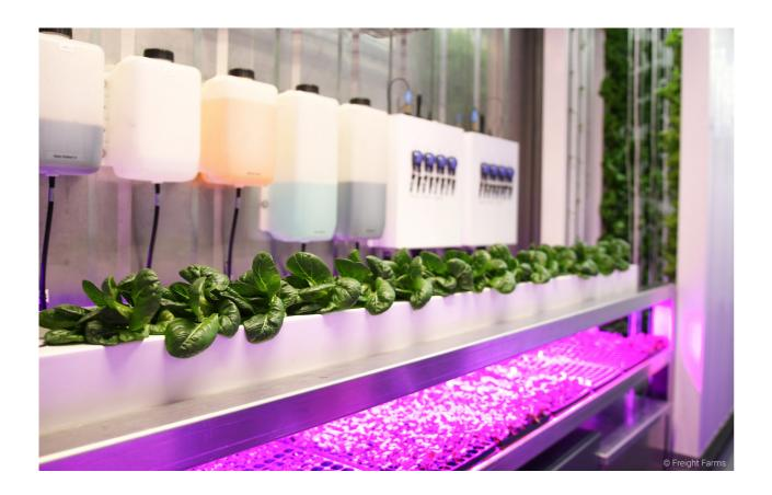
On the contrary of more traditional farming methods, plants grow vertically inside the container thanks to a plug and a constant supply in nutrients, water and LED lights. This independence enables the container farm to avoid the seasonality effect as it would produce under most conditions all year long.
